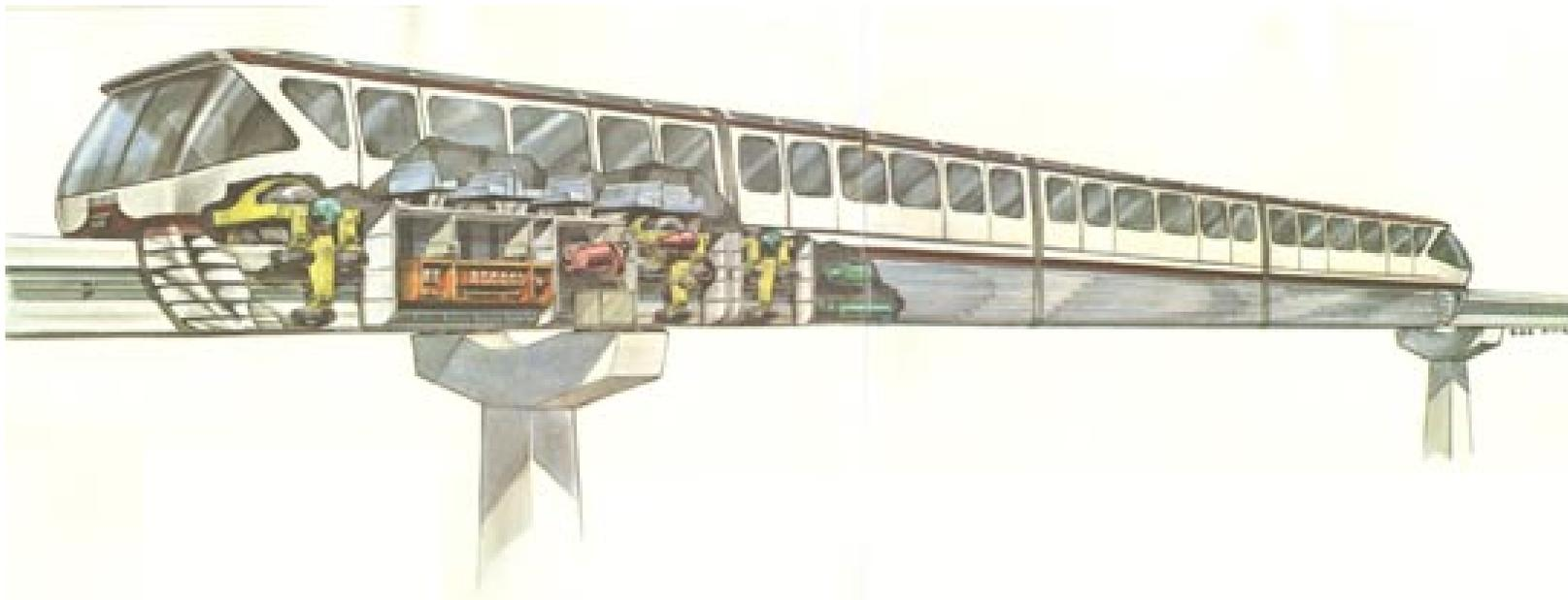
**Top:** A cutaway view of the trains shows the internal transport systems and the rubber tires which propel, guide and stabilize the cars.
